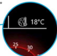
Built-in ambient TEMPERATURE PROBE , essential for temperature compensation during nitrogen pressure testing.
